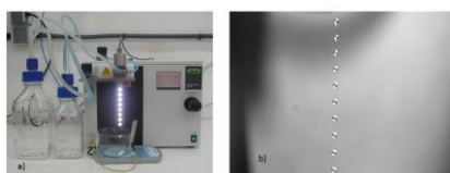
Fig. 1: (a) Encapsulator BUCHI B-390. (b) Formation string of beads with the chitosan (shell) and core material
