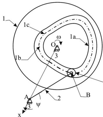
*Fig. 1: Cam mechanism*
