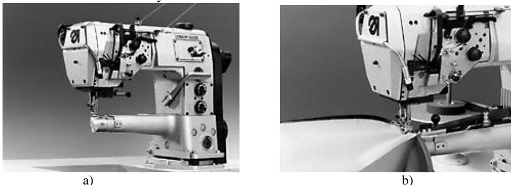
Fig. 5: Cylindrical arm sewing machine: a-general view; b-stitching
