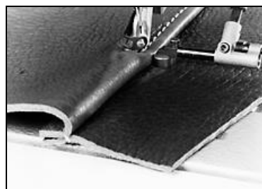
Fig. 12: Restriction device fixed on the machine bed
