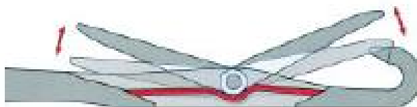
Fig. 1: The schematic positions of the latch needle under the spring action
