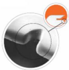
Fig. 9: Deep groove cut in a very short time in sinker platform by abrasive yarns
