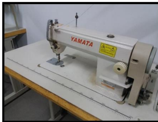
Fig 2. Lock stitch sewing machine
