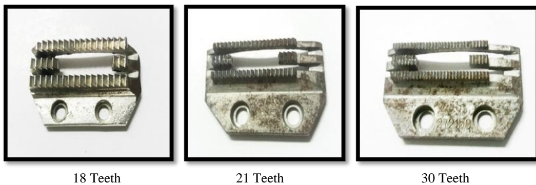
Fig 3. Different feed dogs for three modifications in feed mechanisms
