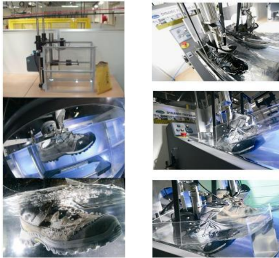
Figure 13: Working diagram for testing final Novadry footwear in static and dynamic conditions
