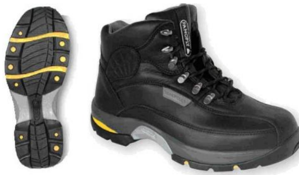
Figure 1: Panoply protective boot, “Multiwalk” design, S3 category: steel 200 J toecap; steel >1100 N sole; damping shock piece, (Panashock); sole’s flexion zones (Panaflex); piece that provides rigidity to the instep (Arch Support System); dual grip and studded outsole; Foot ventilation system
