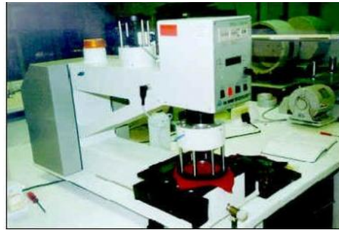
Figure 10 : Smerber water test
