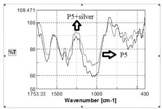
Figure 2. FT-IR spectra for MCT (monochlortriazinyl β-cyclodextrin) treated fibrous composite (P5) and  $P5+[Ag(NH_3)_2]OH$
