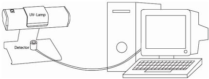
Figure 1: Diagram of UV measurement system.
