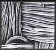
**Figure 5.** Fibre Tencel – fibril and non-fibril appearance
