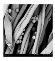
Figure 1: SEM micrographs of cotton fabrics with microcapsules (a) Cotton 1. (b) Cotton 2. (c) Cotton 3
