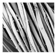
Figure 3: Fibres from the yarns made from the highest possible production rate
