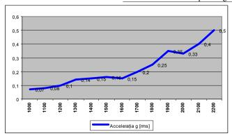
Figure 17. Acceleration amplitude depending on operating mode
