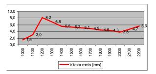
Figure 5. Speed amplitude depending on operating mode
