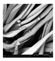
**Figure 2:** SEM micrographs of cotton fabrics after five washing cycles (b) Cotton 1. (b) Cotton 2. (c) Cotton 3
