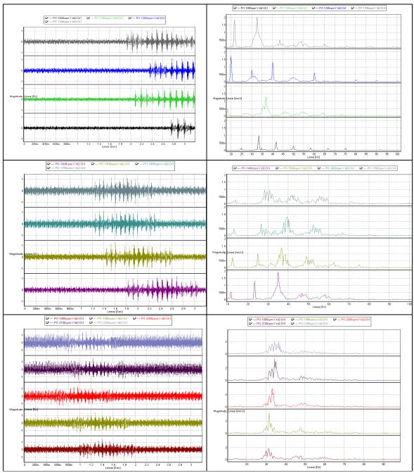
**Figure 13.** Waveforms and frequency spectogramele recorded at the measuring point Pt1 on the horizontal direction measurement
