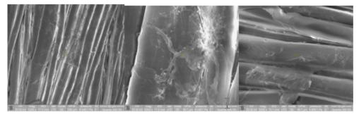
Figure 2: The SEM images for grafted (with cyclodextrin as inclusion complex) flax textiles dyed with redonion and bilberry extracts inspected at different magnifications:(X1200 and X5000)
