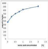
Figure 2: Effect of acetic acid concentration on the value of the capacity factor
