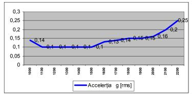
Figure 12. Acceleration amplitude depending on operating mode
