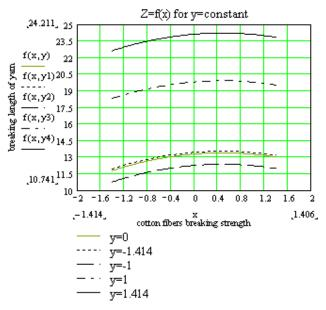
Figure 6. The influence of the cotton braking strength about the breaking length of Nm 40 yarn
