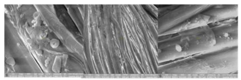
**Figure 1:** The SEM images for reference flax textiles (without cyclodextrin) dyed with onion and bilberry extracts inspected at the different magnifications: (X1200 and X5000)
