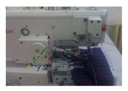
Figure 9. SunStar buttonhole machine with sensor for measuring vibrations installed on the horizontal direction
