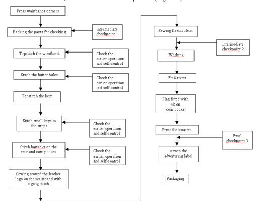
Figure 1. Flow chart for manufacturing process
