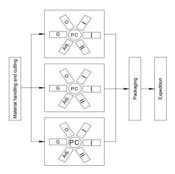
Figure 1. Proposal of cell production for mass custom-made clothing
