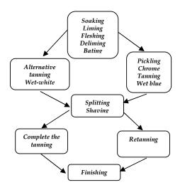
Figure 1. WET-WHITE vs WET-BLUE Tanning Technology Flow Chart
