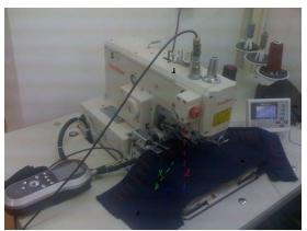
Figure 14. SunStar buttonhole machine with sensor for measuring vibrations installed on the vertical direction
