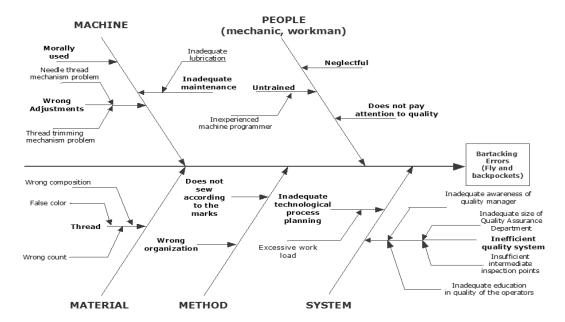
Figure 5. Cause-and-effect chart for the second checking point
