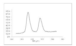
**Figure 3** XPS spectrum of Ag3d in surface of P5 antimicrobial specimen
