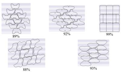
Figure 2: Nesting layouts and material usage coefficient for different footwear parts
