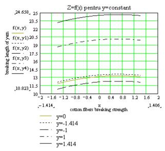
Figure 5. The influence of the cotton braking strength about the breaking length of Nm 34 yarn
