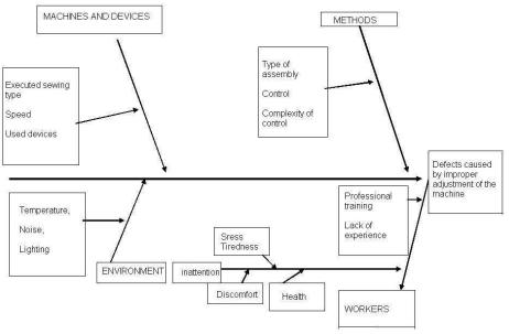
Figure 2. Analysis of the general causes due to the machine
