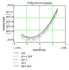
Figure 4. The influence of the polyester ratio about the breaking length of Nm 40 yarn
