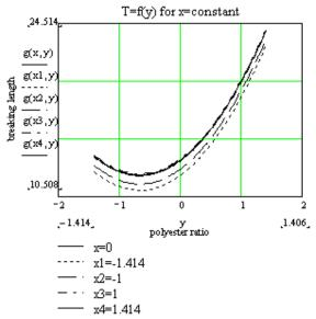
Figure 3. The influence of the polyester ratio about the breaking length of Nm 34 yarn
