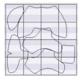
**Figure 1:** Estimation methods for leather products based on parts compact drawing *left* - bounding rectangle method; *right* - squares method
