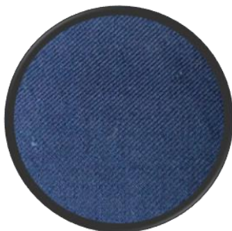
Fig. 1: Cotton knit dyed with azoic dye Direct Blue 6
