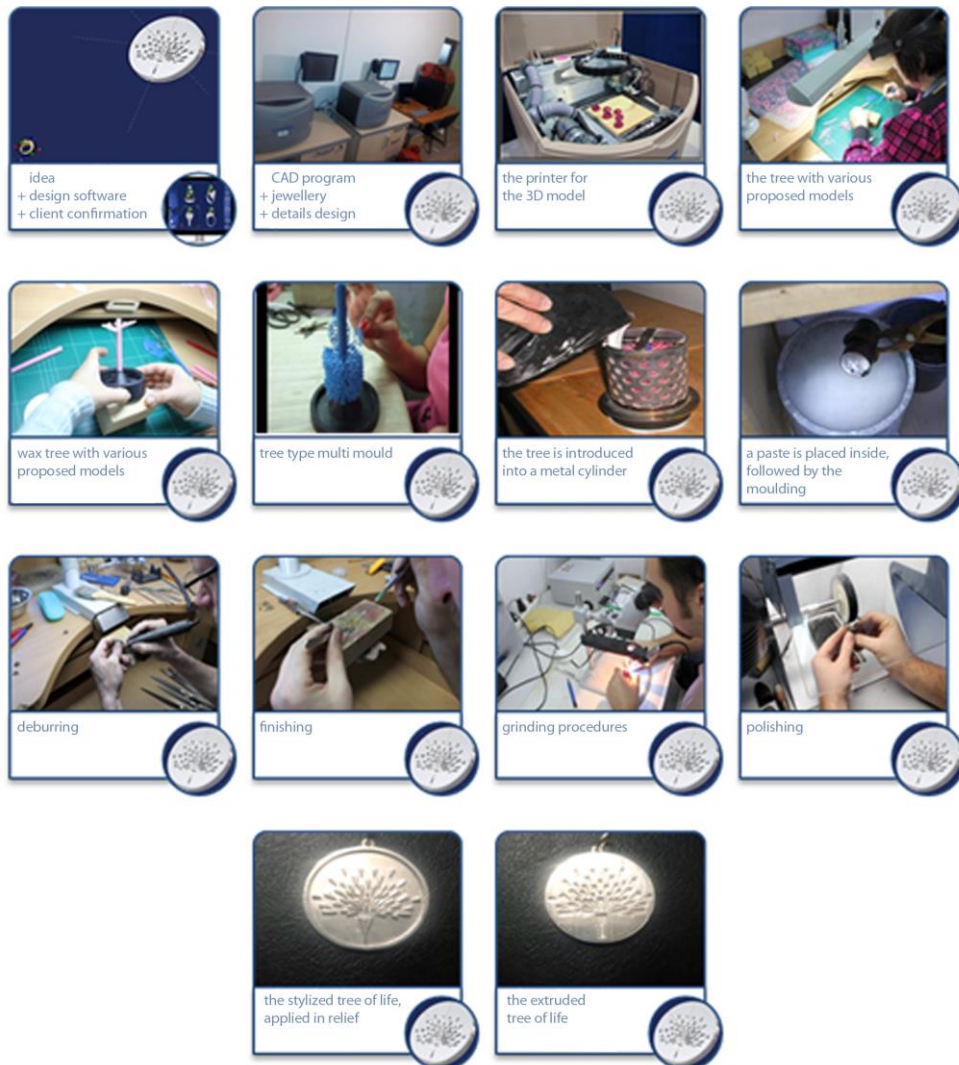
Fig. 6: The way of making a silver pendant with the “Tree of life” symbol. The symbol is made by the designer Negru Diana in relief (in two graphic variants)
