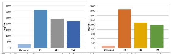
Fig. 2: Flexural stiffness in warp and weft direction of the cotton treated with different types of chitosan
