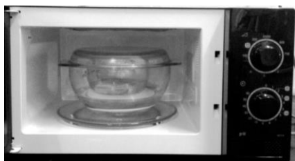
Fig. 1: Reaction vessel inside of the microwave oven
