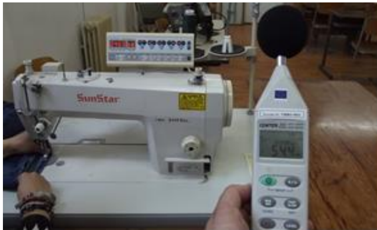
Fig. 1: The measurement of the level of noise of sewing needles for a simple sewing machine
