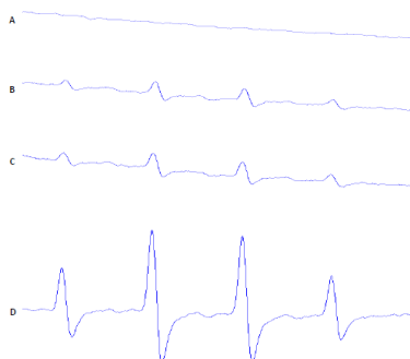
Fig 2: ESR spectra of 100 g/l zinc oxide samples (A: Only DMPO solution, B: DMPO + zinc oxide under dark conditions, C: Pre-exposure of zinc oxide than mixing with DMPO solution, D: UV exposure of DMPO + zinc oxide suspension)
