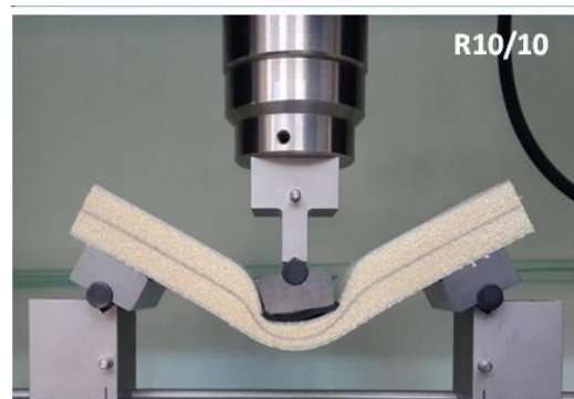
Fig. 4: Force-deflection behaviors of the specimens against bending
