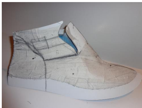
Fig3.a: Fixing the basic design on the last
