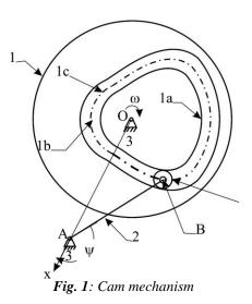
The mechanism presented in fig.1 is composed of: plan cam with groove 1 (bilateral contacts), oscillating follower roll 2 and the framework 3. The contact between the follower and the cam is made by a roll, which go in the groove of the cam.
