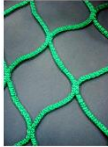
Fig. 3: Net made with double bar raschel machine
