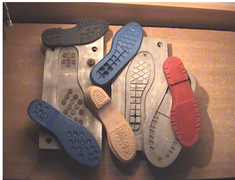
Fig. 4: Mould with assembled modular cavity
