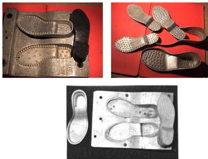
Fig. 3: Modules for cavity forming in moulds with unique cavities
