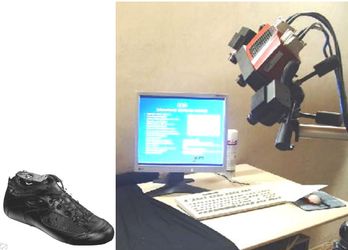
Fig. 3: The copying process in 3 D of the shoe last with the faces pulled with the scanning machine
