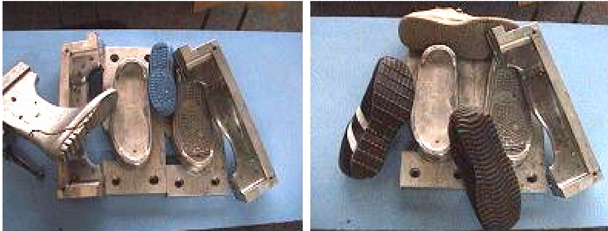
Fig. 7: Mould with modular cavity for sole injection directly on the footwear uppers
