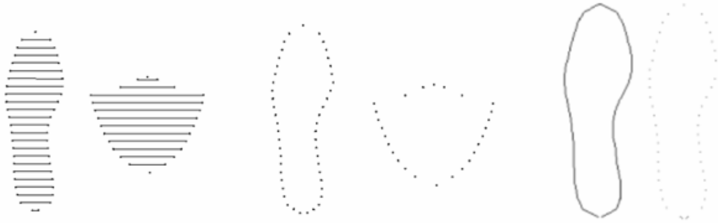
Fig. 1: Discretization of the geometrical shape into a finite number of steps
