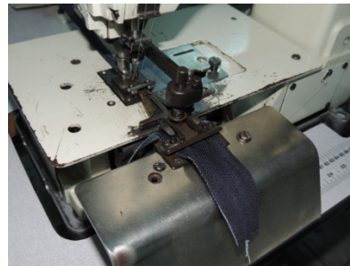
Fig. 2: Driving device and the strip of reinforcement material
