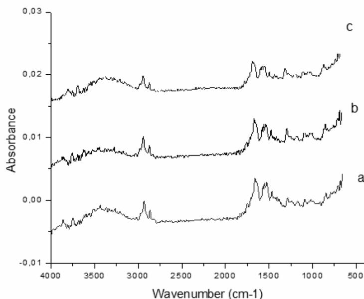
**Fig.5.** Wool IR spectra: a) initial sample, b) ultrasonicated in water for 2h; c) ultrasonicated in TCE for 2h.
