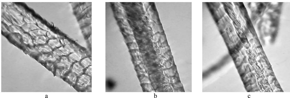
**Fig.2.** Microscopic images of wool samples: a) initial sample; b) ultrasonicated in water for 2h; c) ultrasonicated in TCE for 2h.
