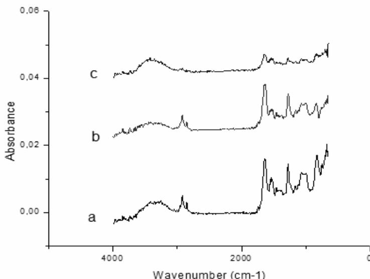
**Fig.4.** Human hair IR spectra: a) initial sample, b) ultrasonicated in water for 2h; c) ultrasonicated in TCE for 2h.
