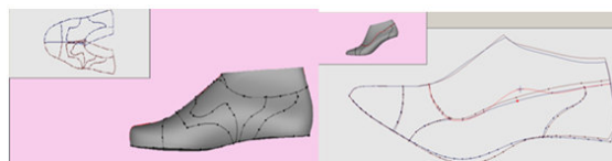
Fig. 6: Using Shoe Design perming the flattening of the shoe last for creating 2D part
