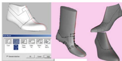
Fig. 5: Creating style-line on the last surface with this 'user friendly' using the session of Shoe Design application
