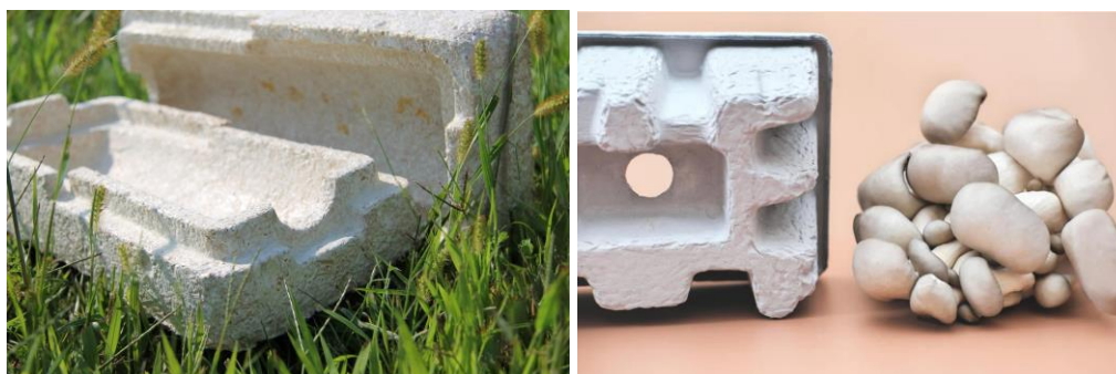
Fig. 1: Mycelium derived packaging materials (Source: www.weforum.org ; www.naturamushrooms.com )
