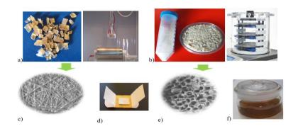
**Fig.1** Images of a, c,d) collagen gelatin from rabbit skin processed by electrospinning in view of wound healing patches manufacturing and b,e,f) lyophilized keratin processed as a porous powder in view of new wound-healing creams or gels fabrication.
