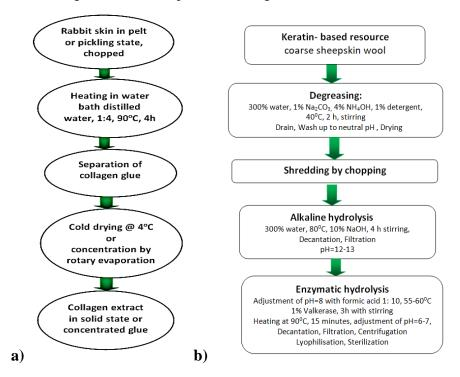
Fig.1: Technology flowcharts of a) collagen and b) keratin extraction and refinery from leather byproducts or coarse wool
