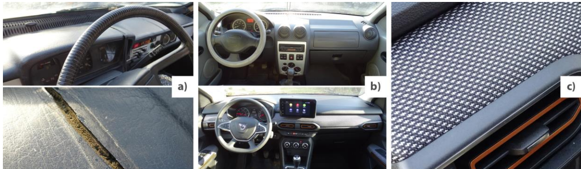
Fig. 1: a) Dacia 1310 dashboard made of polyurethane and PVC foil - damage caused by the overheating of the material during summertime; b) Comparison between a conventional ABS and PVC dashboard (Dacia Logan 1) and an ABS and PVC dashboard with a fabric insertion (Dacia Sandero Stepway 3); c) Fabric insertion - detail (Dacia Sandero Stepway 3)
