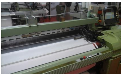
Fig. 1: Rapier loom at SC Majutex SA – Iasi for weaving the fabrics
