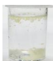
Fig 3: Appearance of the microcapsules at rest for SAMPLE A after 24 h at 37°C.
