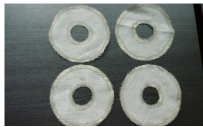
Fig. 2: The fabric variants tailored accordingly to the standard ASTM ES07
