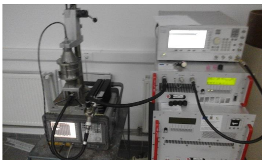
Fig. 3: Electrical device system for measuring the shielding effectiveness
