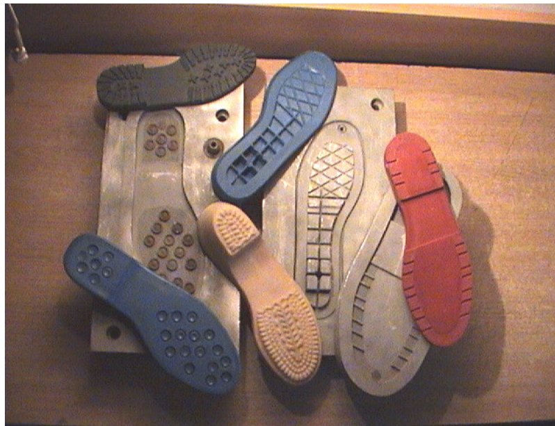
Fig. 4: Mould with assembled modular cavity
