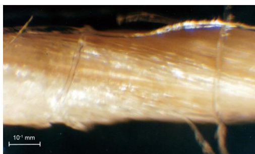
Fig. 1: Longitudinal morphology of a 50% hemp 50% MPP spun yarn (x150 magnification)
